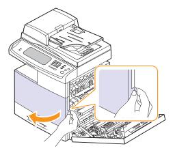
Pull the corresponding toner cartridge out from the machine.
